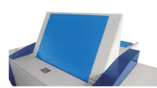
In addition, if the next new plate is set on set table during exposure, the next new plate is loaded automatically just after exposed plate is discharged to the processor.
